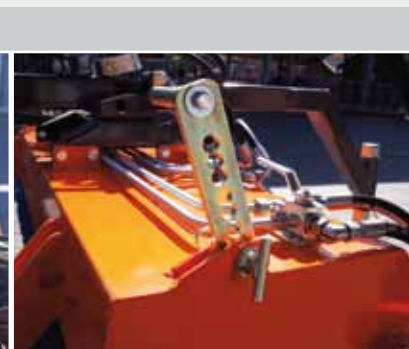
Adjusting-lever system with optimized sweeping-angle
